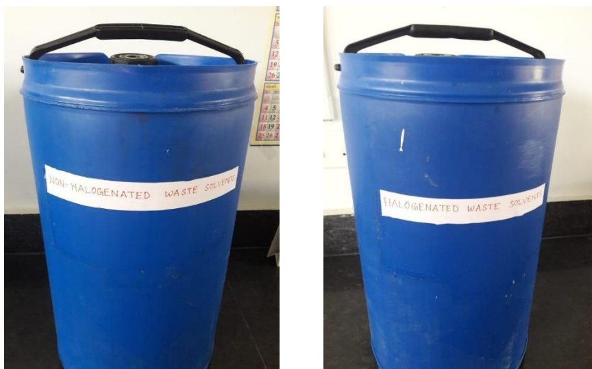
Figure 3: Halogenated and non-halogenated waste solvent drums
